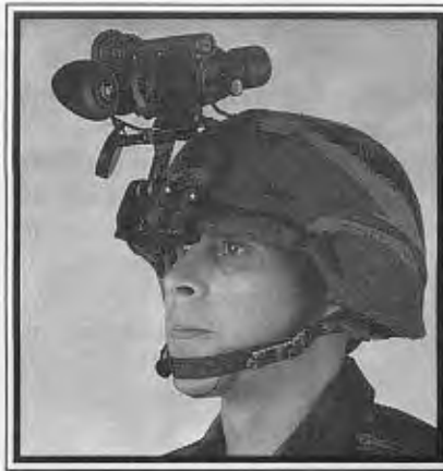
Night vision devices, such as ITT's PVS-7B with flip-up helmet mount, enhance night recon ability, make low-light ops possible. Photo: author's collection
